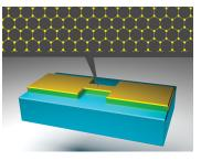
Theoretical Study on High Frequency Graphene|Nanoribbon Heterojunction **Backward Diode**
